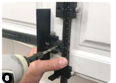
8 Hold securely and drill through fixed center bushing for bottom hole.
