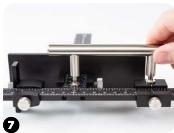
7 Set hardware onto spacing pins and press down until fully seated. Tighten thumb screws to set spacing.
