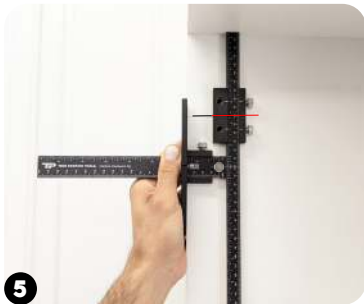
5 Place two Drill Guides side by side to achieve 32mm spacing. Position tool with Large Stop and T-square firmly against cabinet surface. Adjust Drill Guide centers to previous mark and tighten. Drill first set of hinge plate holes.
