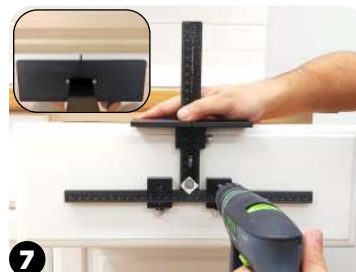
7 Line up notch on Large Stop with mark from Step 4, then drill.
