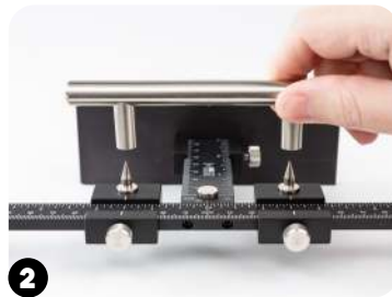
2 Place Hardware Spacing Pins in bushings, keep Drill Guides loose. Set hardware onto spacing pins and press down until fully seated. Tighten thumb screws to set spacing. Ensure measurement is equal on both sides of the jig.
