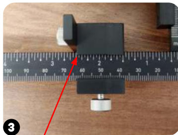
3 Set End Stop to measurement from Step 2 and tighten.
